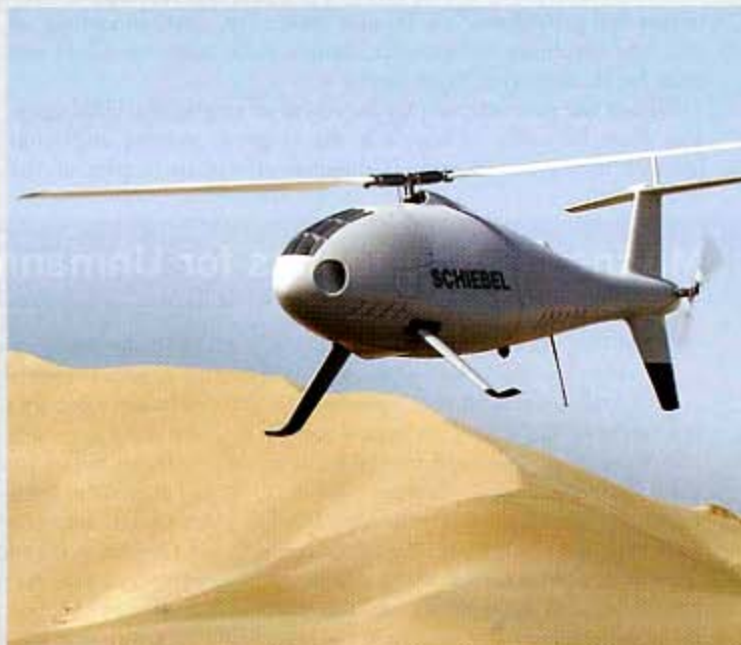
The S-100 vertical take off and landing UAV is under development in conjunction with the United Arab Emirates' UAV research and development center. (Schiebel photo)
