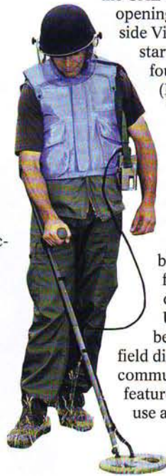
■ The dual-mode ATMID all-terrain metal detector is effective in both normal soil conditions and those with a high content of iron or aluminium oxides. Schiebel: 1130691
