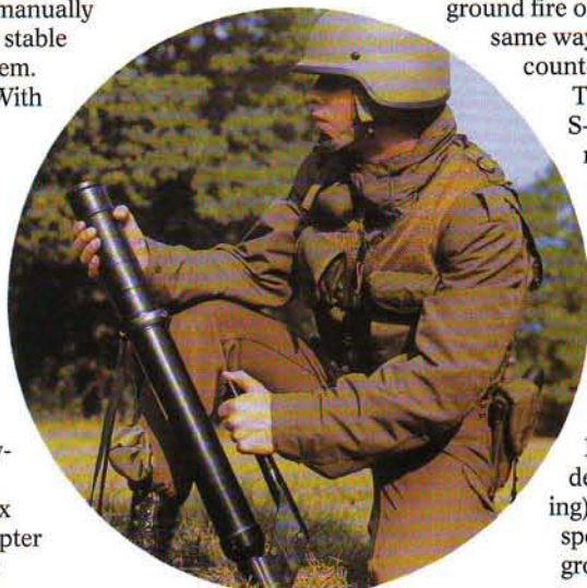
■ The M6C-210 commando mortar has a trigger mechanism for rapid intuitive firing at short ranges, using either elevated or flat trajectories.
