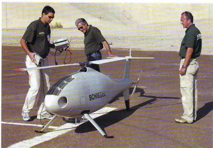
■ A Camcopter S-100 air vehicle is prepared for a test flight without its optronic payload. It can be flown at an altitude of 20,000 ft and with a single relay can be controlled over a 400 km ground-air link, or further still using a satellite connection.
