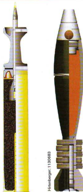
■ Left: Hirtenberger is developing an enhanced version of its APFSDS M57 105 mm medium-pressure round to provide increased lethality for the Kurassier light tank.
