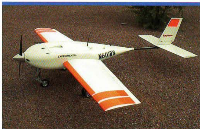
The 3.05-metre wingspan Cobra is powered by a two-stroke, 16.5-horsepower Desert Aircraft engine. It weighs about 20.5 kilos and is 2.75-metres long. (Raytheon)
