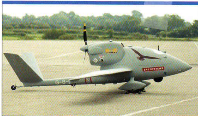
The Herti is based on a Polish motor-glider, the J6 from J&AS Aero design, originally powered by a Honda motorboat engine. However, the Herti flies under the power of a BMW motorbike flat twin, although a Rotax 914 might cut in to increase power. It has a 12.6-metre wingspan and a 5.1-metre length. (BAE Systems)
