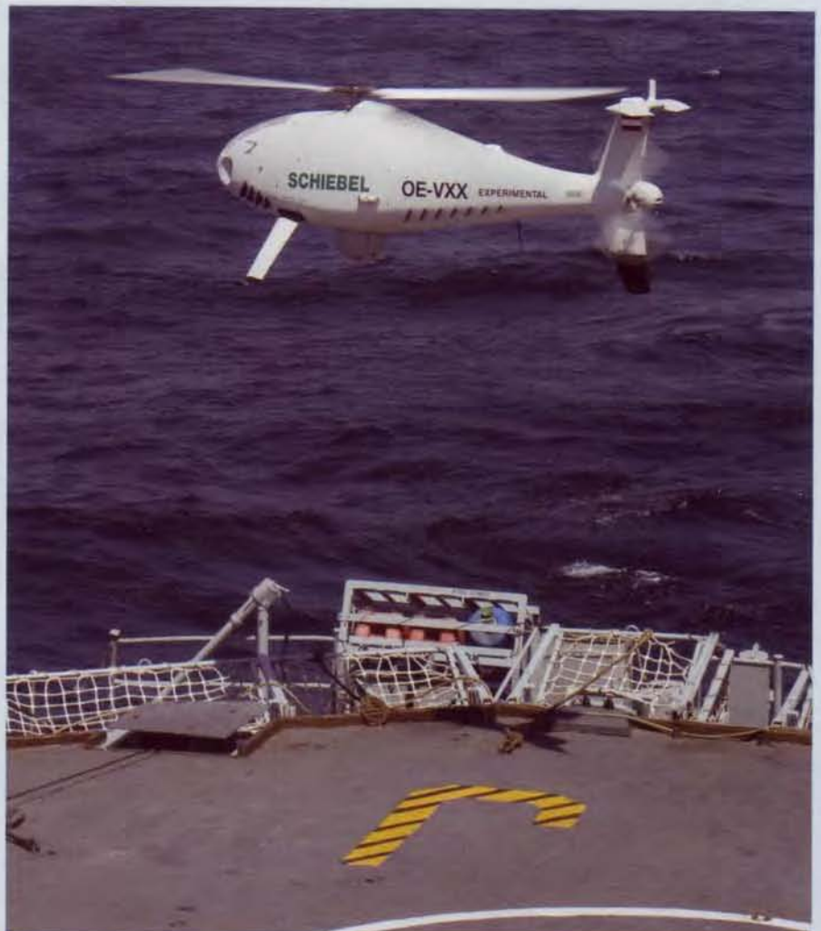
▲ Schiebel's Camcopter S-100 has been demonstrated to a number of navies in the Asia-Pacific region. (Photo: Schiebel)
