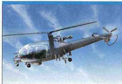
Israel Aerospace Industries' Malat division is developing a naval rotary unmanned air vehicle (Nruav) for the Indian Navy, based on the Hindustan Aeronautics-built Chetak (Alouette III). (Israel Aerospace Industries)
