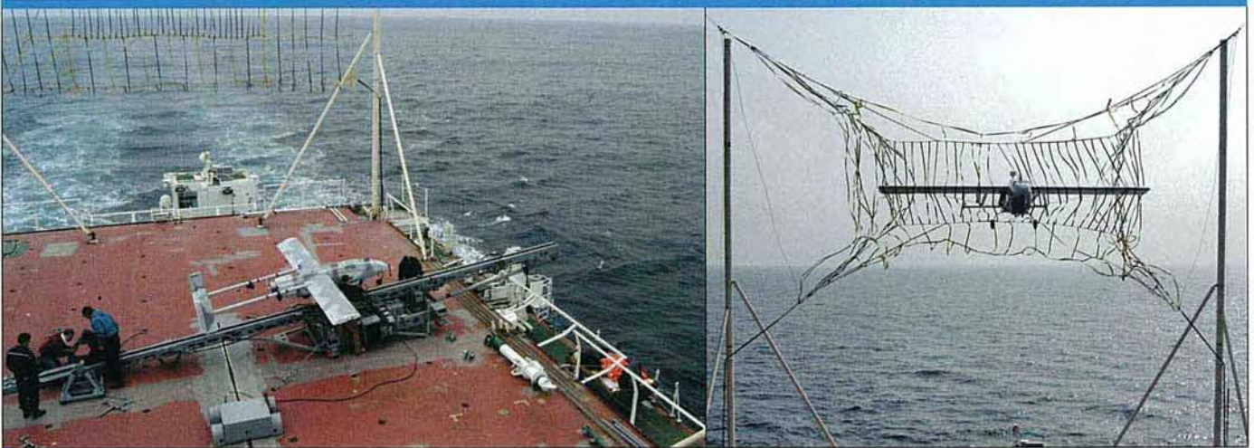
Most ship-based drones are rail-launched, as instanced by this 221-kg AAI Shadow 400 about to depart (left) from the rear deck of a Republic of Korea Navy vessel. Recovery is performed by remotely piloting the drone into a large vertical net, a technique developed for the same manufacturer's RQ-2 Pioneer. (AAI)
