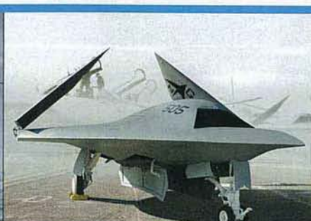
Naval unmanned combat air systems are being pioneered by Northrop Grumman, funded to produce and test two X-47Bs under the US Navy's Ucas-D demonstration programme. The US Navy needs to establish with the X-47B that a Ucas is compatible with the cycle of manned aircraft operations, can be correctly manoeuvred on deck and can be landed safely. (Northrop Grumman)
