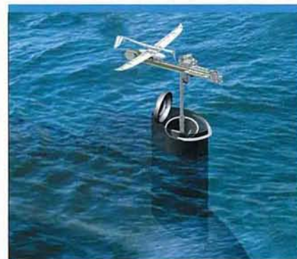
The Volans concept, being developed by EMT and Gabler, would house an Aladin drone and rail in a mast-mounted container, allowing a submarine to launch from periscope depth. (Gabler/EMT)
