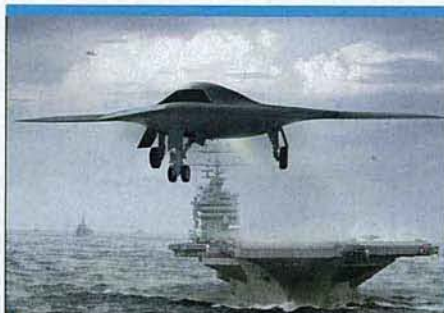
Naval unmanned combat air systems are being pioneered by Northrop Grumman, funded to produce and test two X-47Bs under the US Navy's Ucas-D demonstration programme. The US Navy needs to establish with the X-47B that a Ucas is compatible with the cycle of manned aircraft operations, can be correctly manoeuvred on deck and can be landed safely. (Northrop Grumman)
