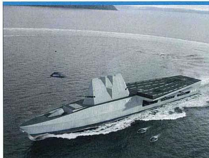
In 2007 BAE Systems released preliminary details of its proposed 8000-tonne UXV Combatant ship, designed to operate large numbers of fixed- and rotary-wing drones for extended periods. (BAE Systems)
