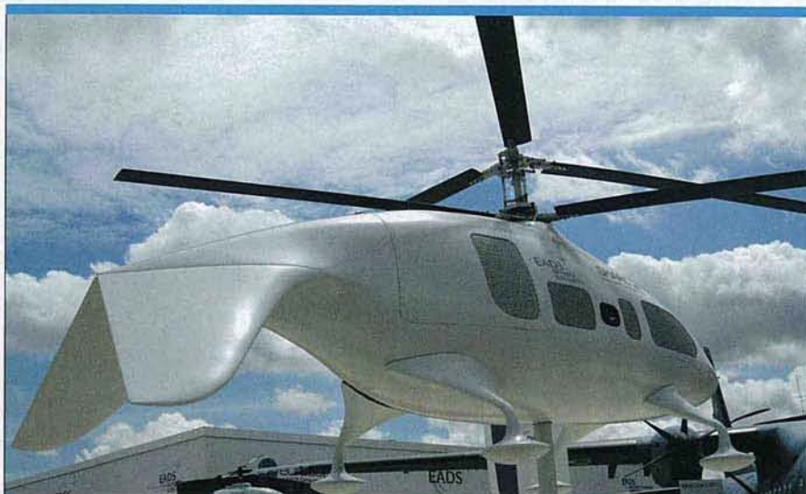
Reverting to a co-axial rotor system derived from that used on the Dornier Seamos radar platform, the 190-kg Eads Sharq is designed to operate from small vessels. (Eads)
