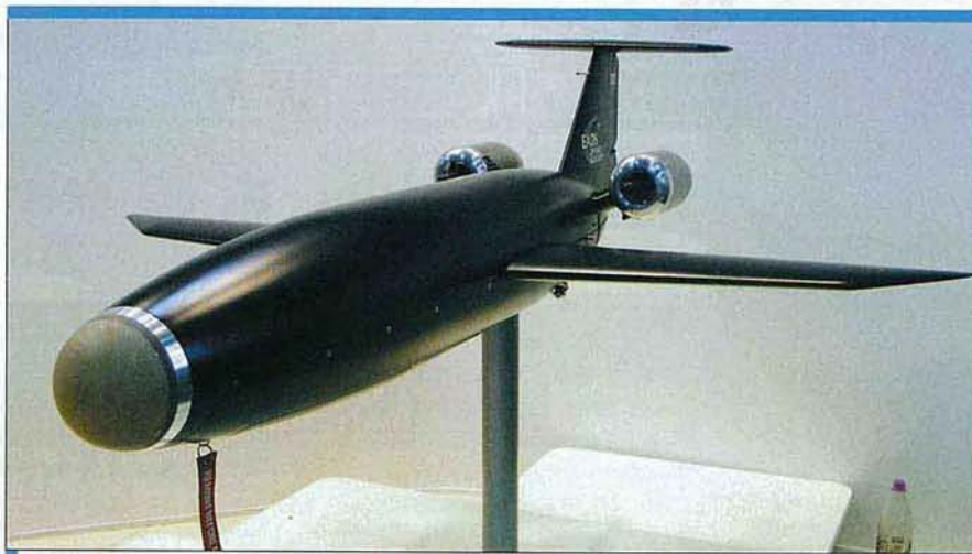
An Eads Do-DT45 IR target with patented 'hot-nose' was used as a target for a South African Navy Denel Umkhonto missile during exercise 'Good Hope III' in March 2008. (Armada/RB)
