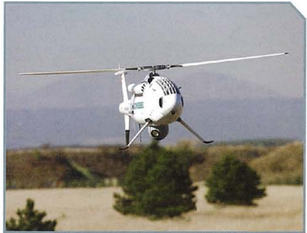
Schiebel's VTOL CAMCOPTER S-100 can be outfitted with special sensors to detect improvised explosive devices (IEDs).
