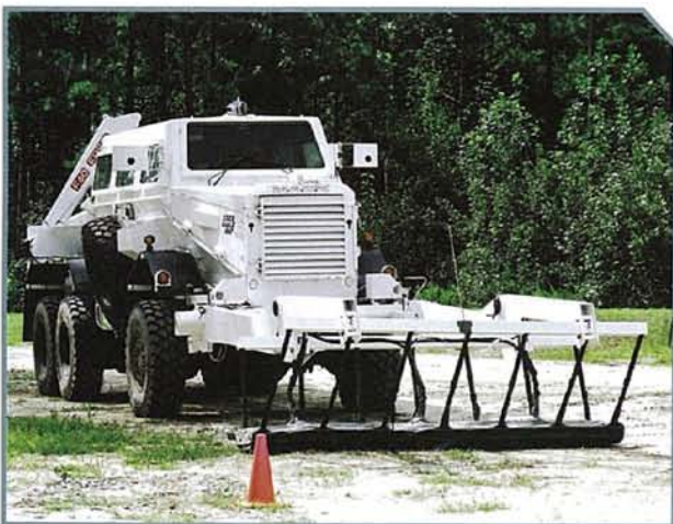
VAMIDS is a versatile, vehicle-based detection and marking system.
