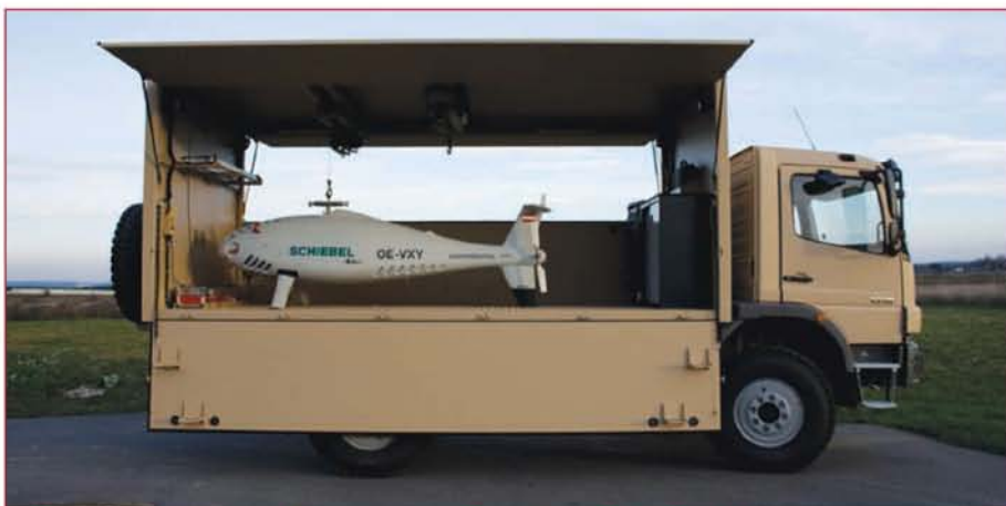
Camcopter shown in one of its transport configurations. (Photo: Schiebel)
