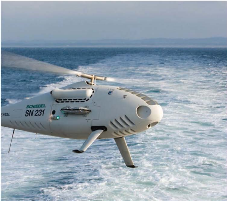
Camcopter seen transitioning out of the hover from a ship while under way. (Photo: Schiebel)
