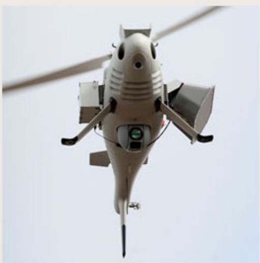
Schiebel offers the S-100 as a versatile multi-mission platform. This Psychological Warfare configuration includes an EO/IR payload for situational awareness, public address (loudspeakers) and remotely controlled magazine for dropping leaflets on demand. Photo: Schiebel Group
