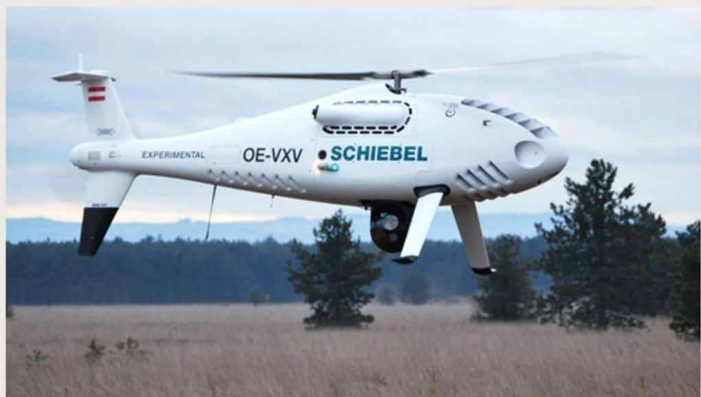
Camcopter S-100 flies with the Wescam MX-10 EO/IR payload. Photo Schiebel group
