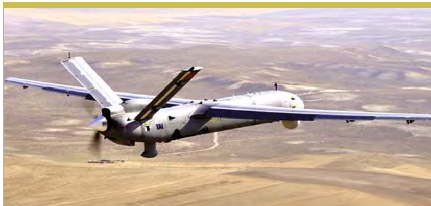
A newcomer on the male scene is the Turkish TAI Anka. The 1.6-tonne, 24-hour endurance drone is expected to enter service in the latter part of 2012. (Turkish Aerospace Industries)
